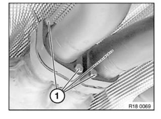
Release screw connections (1) between catalytic converter and rear mufflers.
